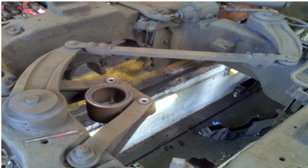
FIG 7 How the Class 66 leading and intermediate axles steer
