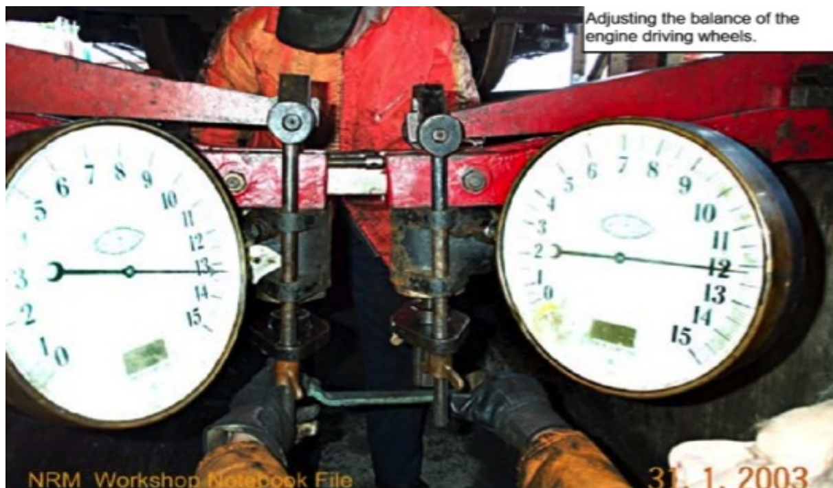
KELBUS SCALES in use on Green Arrow at NRM after changing a spring.
