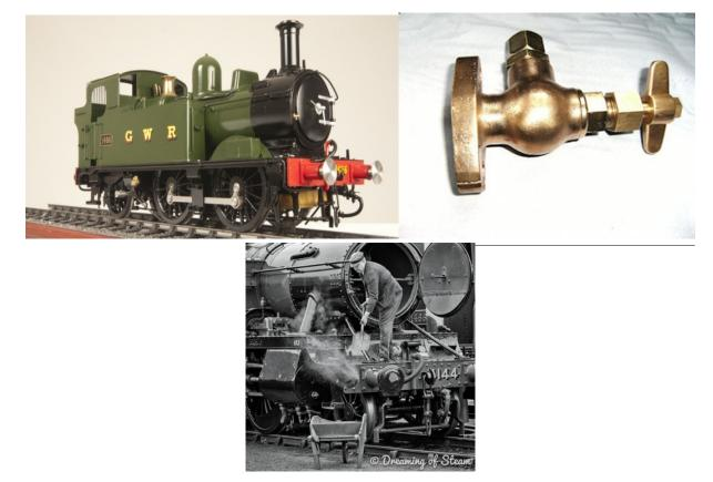
In order to help cleaners and firemen get their locomotives ready and dispose them at the end of the day there was a fitting on the lower right hand side of the smokebox which was connected to the boiler pressure by a pipe inside the smokebox. This allowed the crew to attach a steam lance on the end of flexible piping so as to be able to loosen and clean some of the soot and debris from the parts in the smokebox before shovelling it out.
