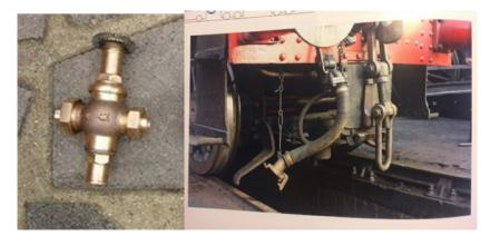
Locomotives fitted with steam heating apparatus are generally equipped with a Mason Valve, generally low down on the footplate. The valve limits the pressure of steam that is drawn off the locomotive's system by means of a pressure-reducing valve. The steam is fed to the carriages in the train through steam heating pipes, which are equipped with, shut off cocks. The hoses should be hung on the hooks provided so that the steam heating hose does not sustain damage from hanging down
