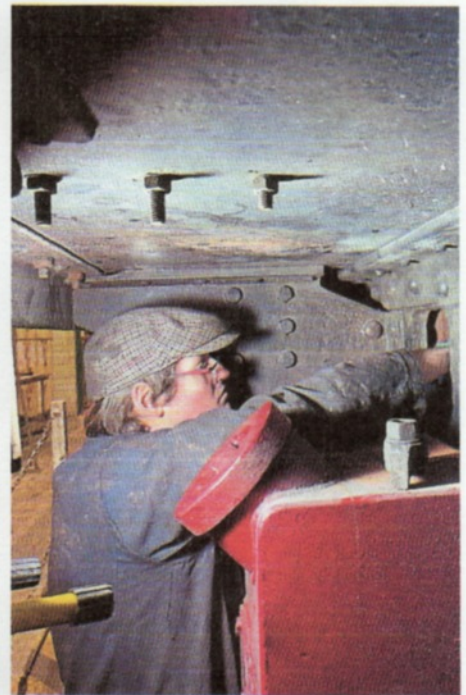
Practical: Tom fits a mudhole door with a new door joint. DAVID GRINDLEY
