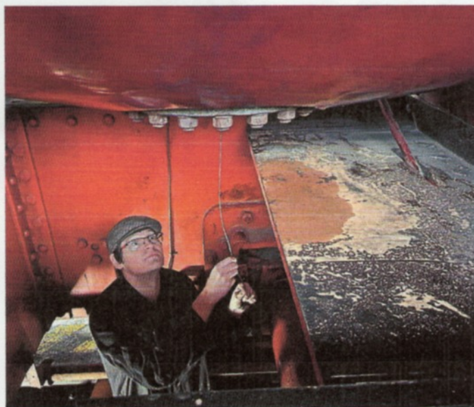
Benjamin removes fusible plugs for inspection. DAVID GRINDLEY
