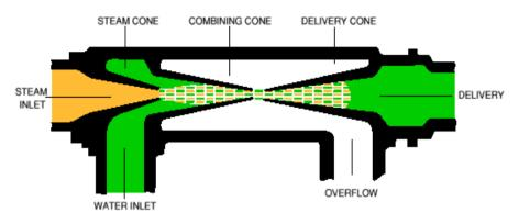
The steam cone directs high temperature steam at high velocity into the assembly. It has a small bore at the tip which restricts the amount of steam coming through. This means that once started, the injector can usually be allowed to run with the steam inlet cock fully open. As the steam passes along the steam cone, a proportion of the heat energy is transferred to giving the steam a high velocity.
