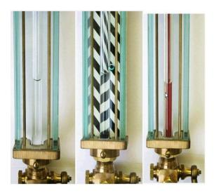
Tube type gauge glasses. Note the heavy gauge glass protector.
