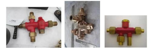
Some of the injectors have integral clack (one-way) valves but in the same way as the feed pumps, it is important to fit a steam-rated one way valve between the injector and the boiler in addition to the isolation cock on the boiler.
