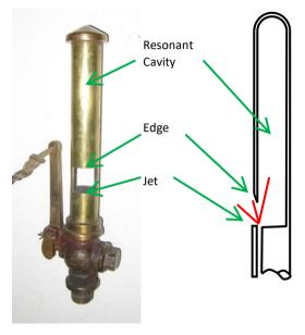
The resonant frequency depends mainly on the length of the tube but the note can jump an octave if higher pressure steam is used. Some whistles have the facility for adjustment of the distance between the jet and the edge which will allow for refinement of the note and volume for the steam plant's normal working pressure.
