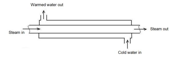
By running in counter-flow the temperature of the water is elevated to closer to the temperature of the steam entering the exchanger. Efficiency of these exchangers depends upon many factors, but particularly internal surface area.
