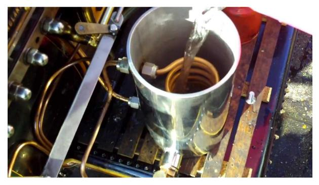
Most kettles are sized between 1 and 2 litres (1½ to 3 pints) and will boil in a couple of minutes when provided with steam at around 7 bar (100 psi). This implies an equivalent power of around 3 kW (4 horsepower) - much the same as the boat's engine. However the kettle is near 100% efficient, while the engine is more likely to be 5 to 10% efficient, so in fact the engine will use much more steam. Even so, the pressure usually drops significantly when the kettle is put on to boil.
