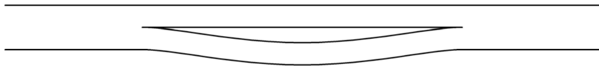
Bulging of the plate due to overheating
