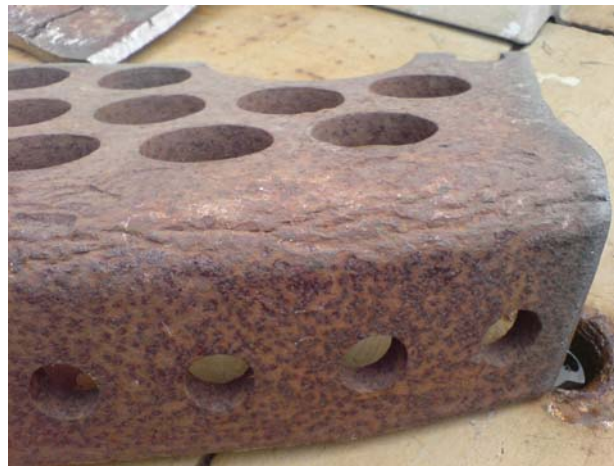
Front tubeplate radius showing cracking caused by stress corrosion.
