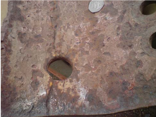
Cracks in a backhead radius, this type of cracking cannot be repaired by welding
