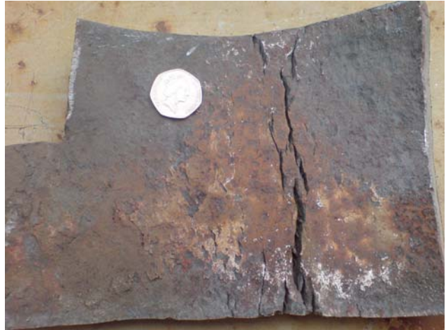
The same radius pressed flat to show the severity of the cracking
